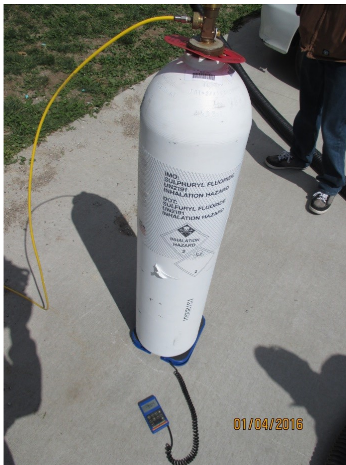
Figure 4.10 The amount of SF applied to the silo was measured by placing the cylinder on a digital scale, opening the cylinder valve to allow gas to flow, and closing the valve when the correct amount of SF had been applied.
