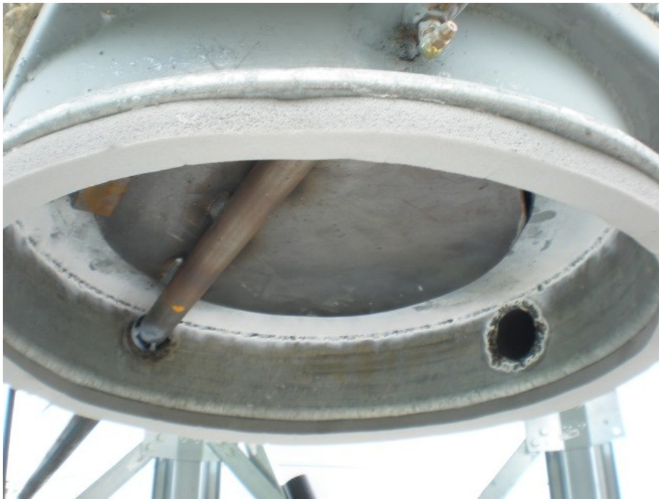
Figure 4.5. Butterfly valve and exit points for fumigant inside \text{PH}_3 reaction chamber.
