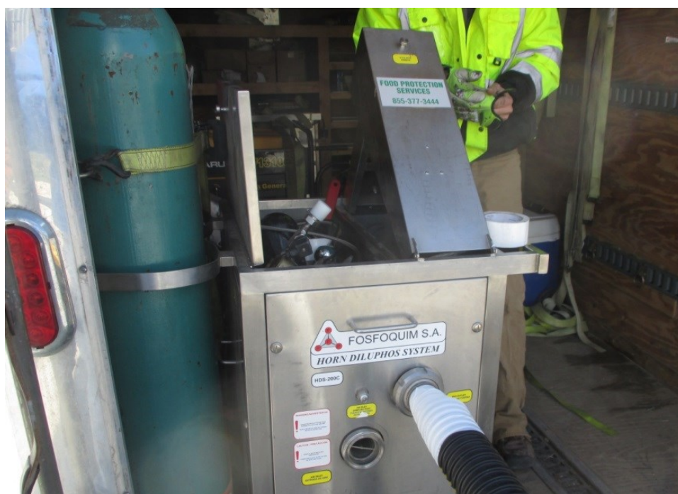
Figure 4.8. Horn Diluphos System used to blend PH 3 and air prior to silo fumigation during trial 4.
