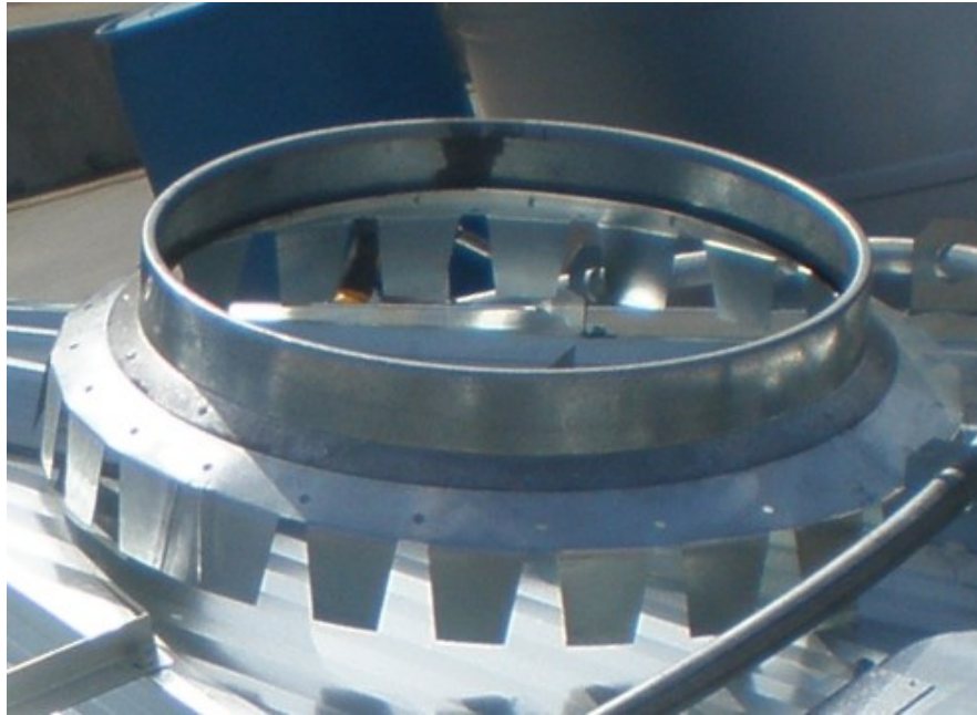
Figure 3.12 Lid from Bird’s Silos and Shelters installed on the SCAFCO “bottle cap” lid section. The thicker, round-edged lip allowed for an airtight fit with the foam strip installed on the underside of the cap (not shown).
