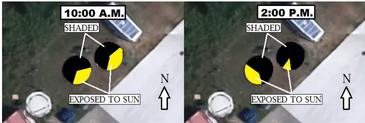
Figure 4.20 Top view of the two silos while under fumigation. The sides of the silos with the lowest gas concentration were shaded throughout most, or all, of the day, and the sides with the highest gas concentration were exposed to more solar radiation unless the sky was overcast.
