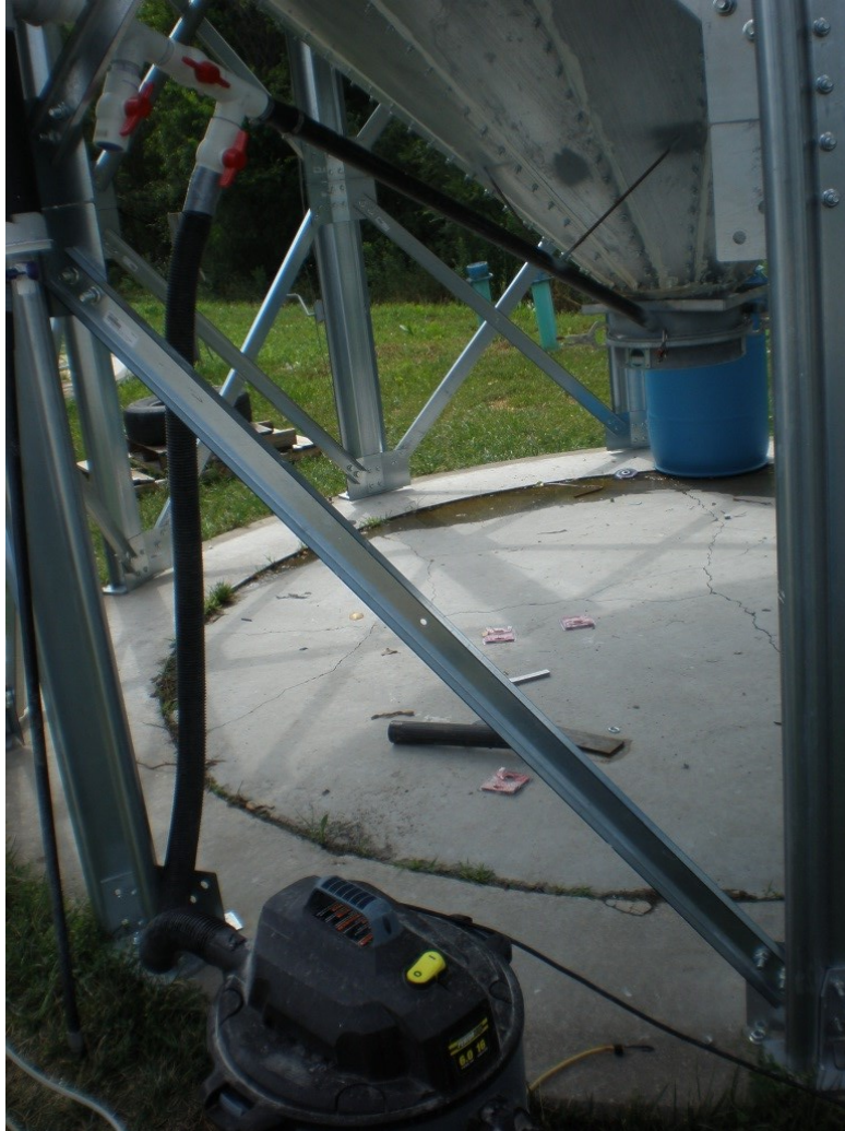
Figure 3.4 Vacuum cleaner set on “blow” connected to ball valve and pressurizing one of the two sealed silos during a pressurization test.
