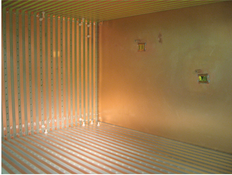
Figure 3.13: A look inside the TPC. The solid copper sheet is the cathode plane and the copper strips lining the TPC are the field cage rings. The TPC frame (i.e. what the copper is attached to) is composed of G10. Figure from Ref. [75].
