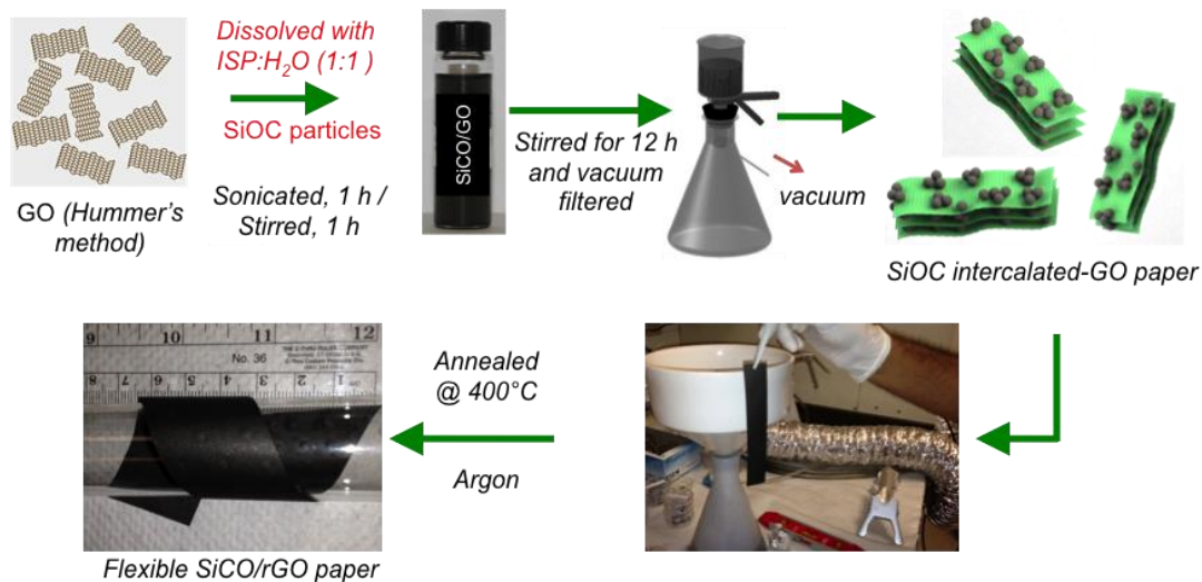
Figure 5-3 Electrode design and fabrication. Schematic illustrating the procedure for fabrication of free-standing SiOC/graphene composite paper for use as Li-ion battery anode. The composite paper was sufficiently robust to be handled by hand and flexible enough to be rolled on to a cylinder several times without breaking.
