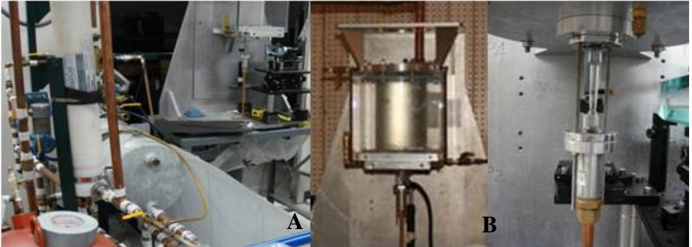
Figure 2.3 Shows A. Test rig, B. Water reservoir, C. Nozzle setup
