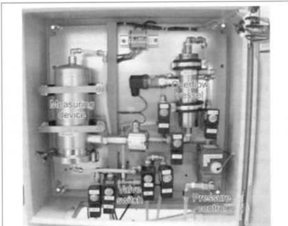
Figure 2: Water intrusion test (final prototype) consisting of a measuring device with a pressure transducer, overflow vessel, valve switch and pressure control.
