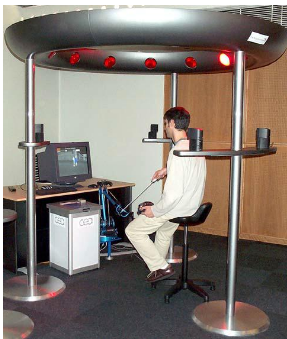
Figure 2.9 HOMERE multimodal system for virtual environment navigation for persons blind or visually impaired.
