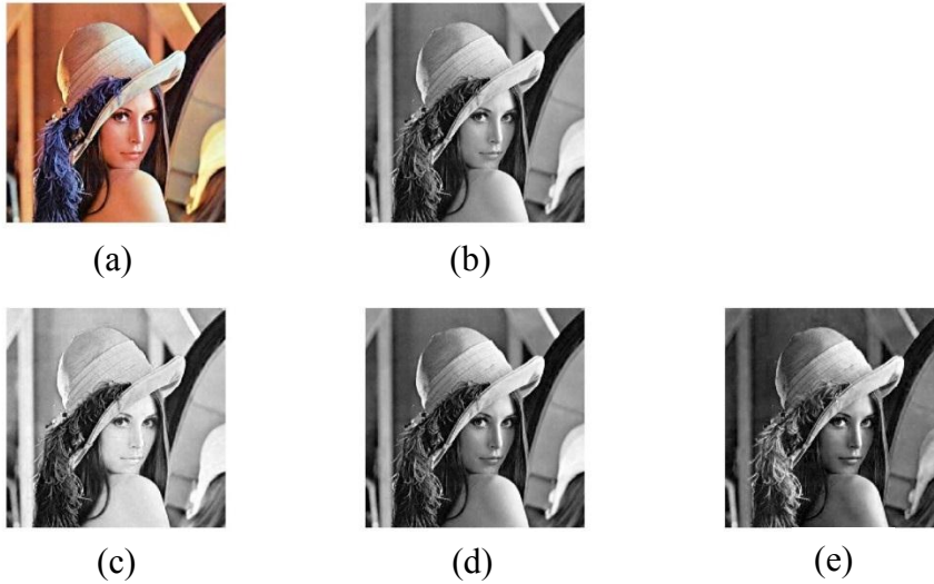
Figure 2.5 Examples of color image to grayscale conversion. (a) Original image; (b) Converted grayscale image; (c) Red channel; (d) Green channel; (e) Blue channel.
