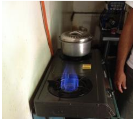
Figure 3.7: Research center cook stove with air mixing
