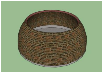
Figure A.13: Building up the lower dome
