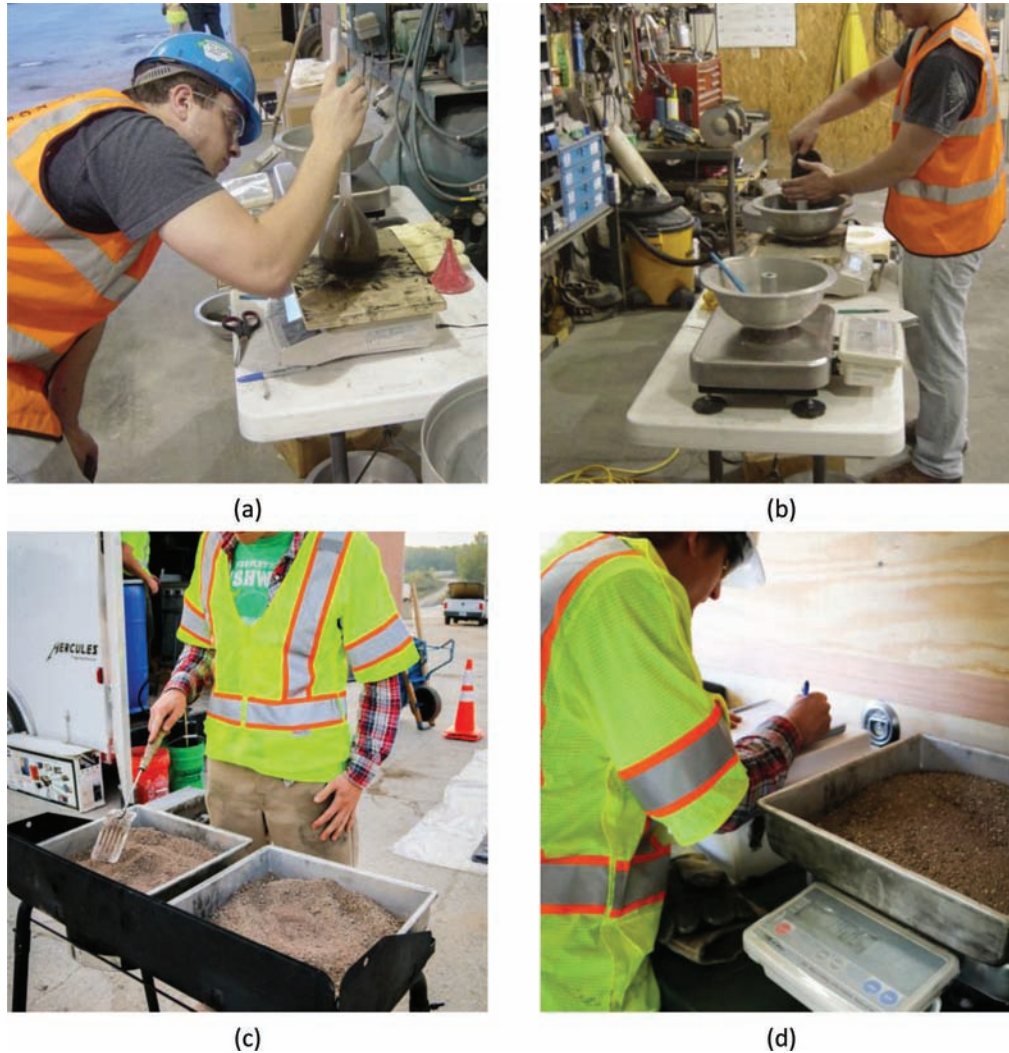
Figure 5.2 Testing of fine lightweight aggregate for use in an internally cured high performance concrete mixture, showing (a) specific gravity testing, (b) ITM 222 centrifuge method, (c) obtaining an oven-dry sample, and (d) measuring oven-dry mass.
