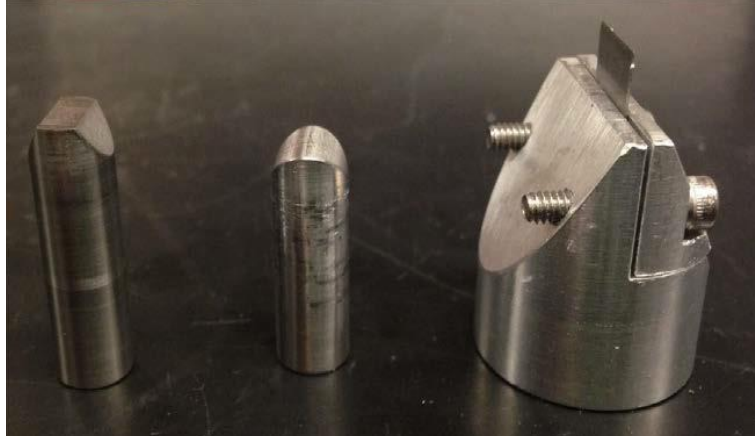
Figure 9: Indenters used in experimental testing. From left to right: FSP, round, and razor blade [13].
