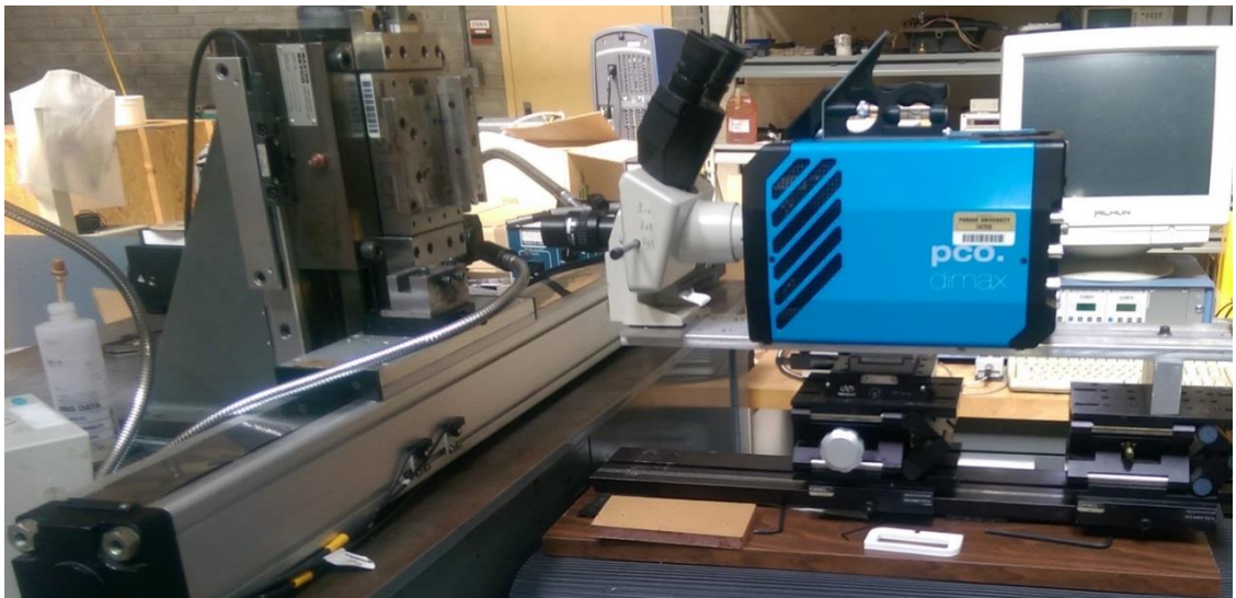
Figure 4.10: Photograph of PIV setup. High speed images are recorded by the camera viewing the cutting process from the side, that is, parallel to the cutting edge
