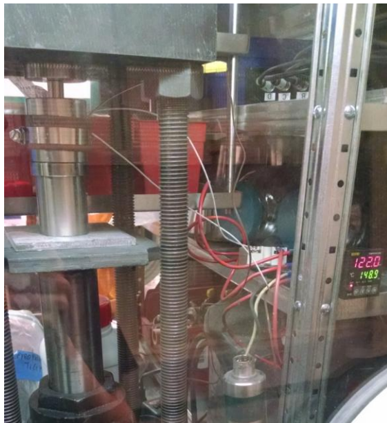
Figure 2.6. Hot press setup in an inert atmosphere (Ar).
