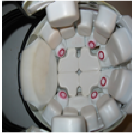
(a) The HITS system within a helmet, the red sections show where the sensors are located within the helmet padding.
