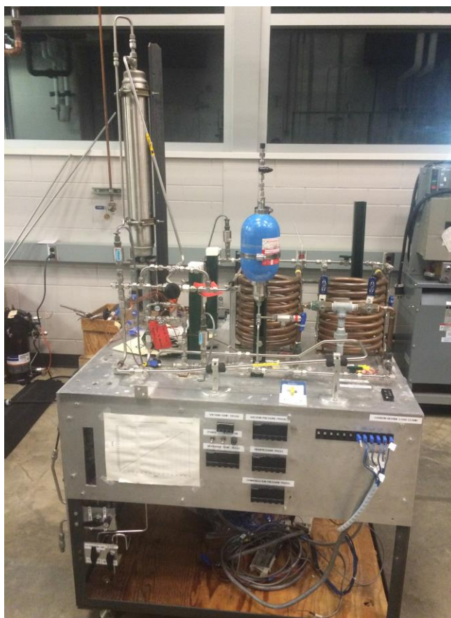
Figure 2: Closed loop system test stand
