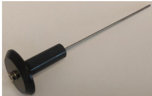
Figure 2: Valve body with attached LVDT armature
