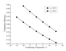
Fig.7 Influence of condensing temperature on volumetric efficiency
