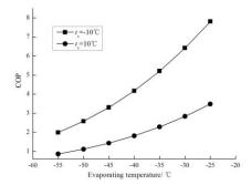
Fig. 11 Influence of evaporating temperature on COP
