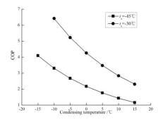
Fig. 10 Influence of condensing temperature on COP
