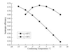
Fig. 8 Influence of condensing temperature on isentropic efficiency
