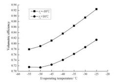
Fig. 6 Influence of evaporating temperature on volumetric efficiency
