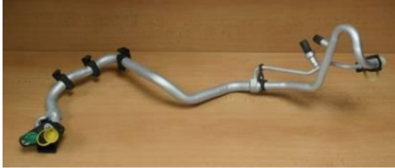
Figure 1: Typical Coaxial IHX
