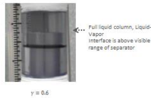
Figure 8: Separator 2, P = 115 Psia [800 kPa] m_T = 6 lbm/hr [2.7 kg/hr]
