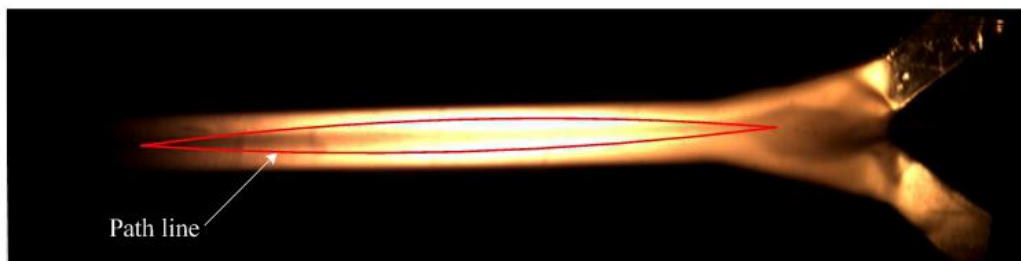
Figure 9: Path line in mixing chamber
