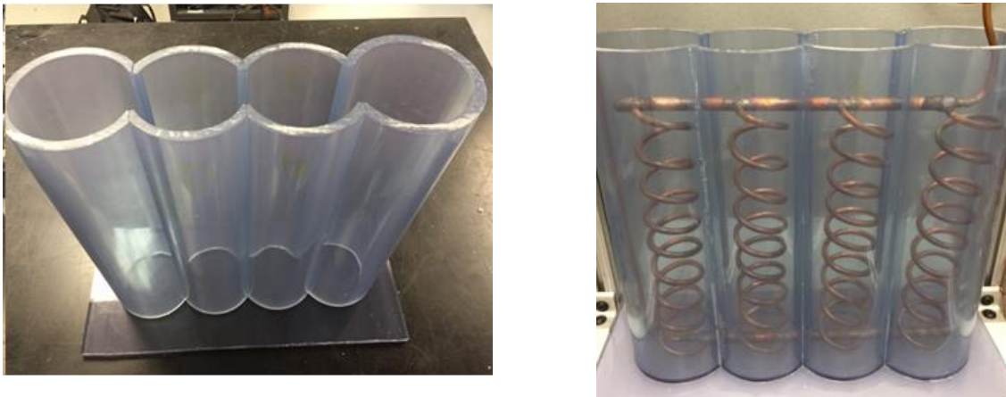
Figure 2: Condenser made from spiral tube placed inside PCM container
