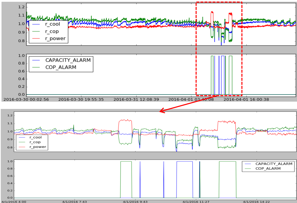
Figure 16 Results of AFDD Field Evaluation on 7.5 ton RTU
