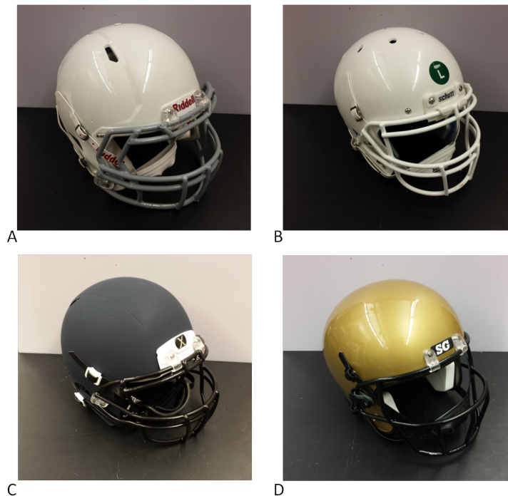
Figure 5.1. Four helmet models were used in this study: A) Revolution Speed (Riddell; Rosemont, IL), B) AiR XP PRO (Schutt; Litchfield, IL), C) X2E (Xenith; Lowell, MA), and D) SG (SG Helmets; Brownsburg, IN).
