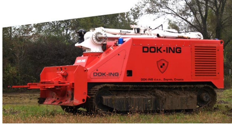
Figure 2.3.: The DOK-ING MVF-5 firefighting robot (“MVF-5”, n.d.)
