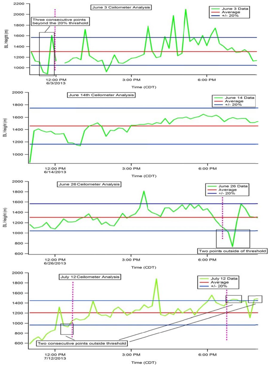
Figure 3.5 – Ceilometer data for each case study day from the SOAS campaign. The red horizontal line establishes the afternoon average, and the blue lines represent \pm 20\% deviations from the mean. Vertical dashed lines define time cut off points.
