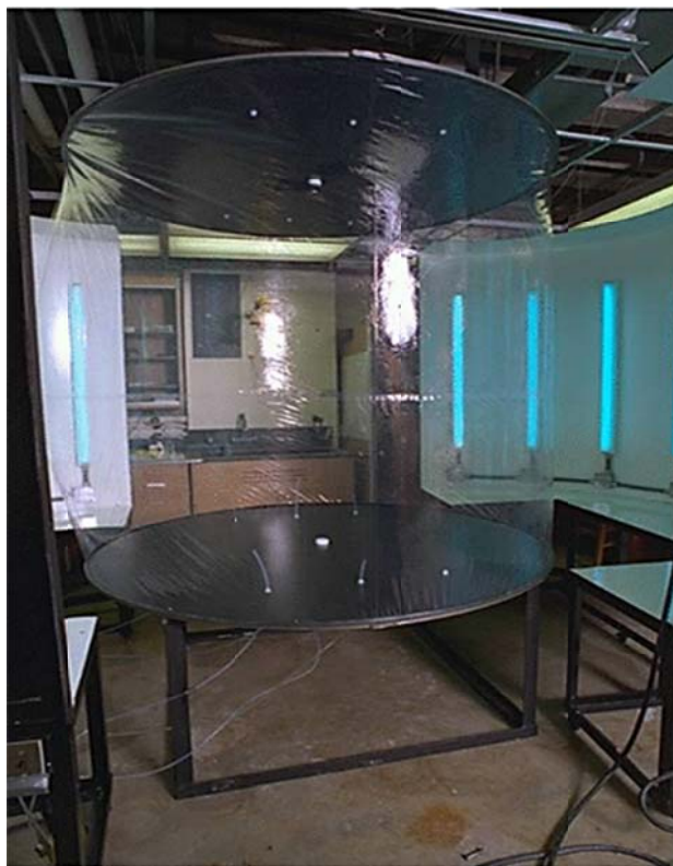
Figure 2.1 – Image of photochemical reaction chamber used for the May 2013 experiment [Costa, 2010].
