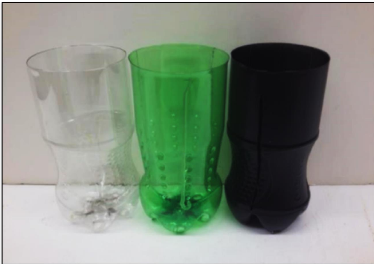
Figure A11. Comparison of three opacities (clear, green, black; left to right) and three spiral control techniques (control, internal ridges, side-slits; left to right) in Bottle Modification Experiment.
