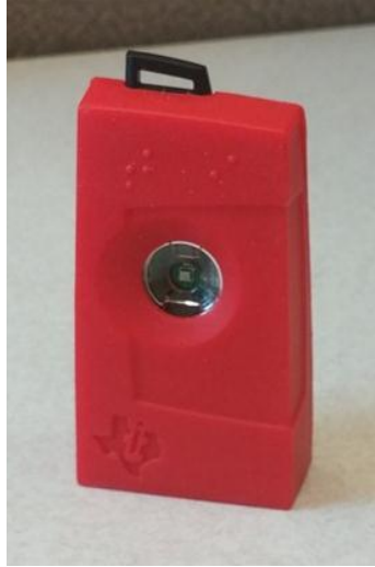
Figure 2: Texas Instruments CC 2541 Sensor Tag (approximately actual size).
