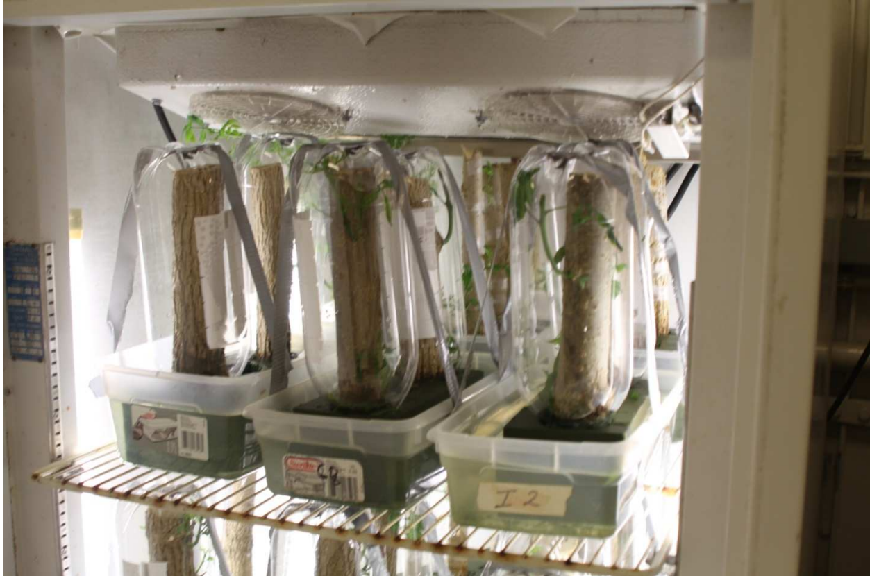
Figure 3.1 Ash bolts in floral foam with two liter bottles in the laboratory 2014.
