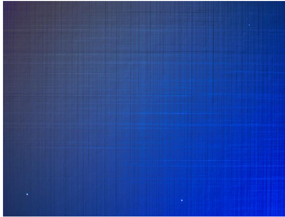
Figure 2.19. Nomarksi contrast optical micrograph of a wafer showing so-called cross hatch morphology. The field of view is \sim 2.5 mm wide.
