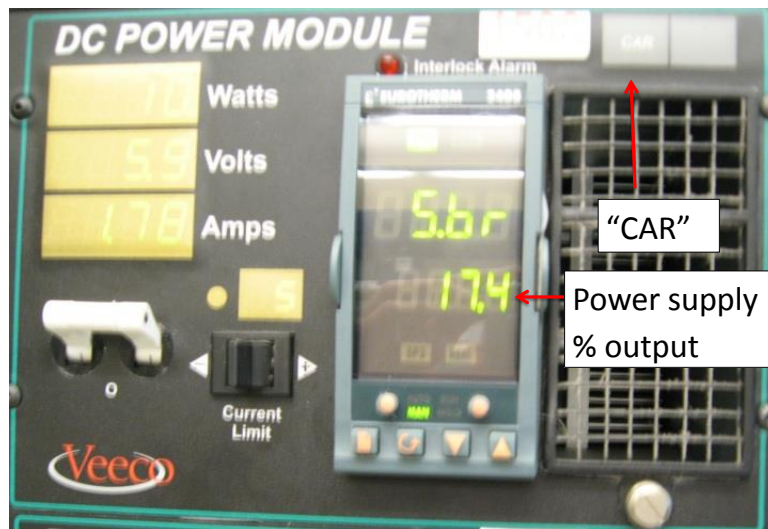
Figure B.3. Check the power output % as soon as you start ramping the CAR heater.
