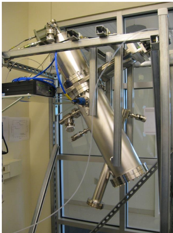
Figure 2.17. Dedicated gallium outgassing chamber. The chamber featured a near-vertical port to enable the the crucible to be filled almost completely with gallium. The frame supporting the chamber could be rolled into position next to the MBE to allow sources to be passed into the MBE without exposure to air.
