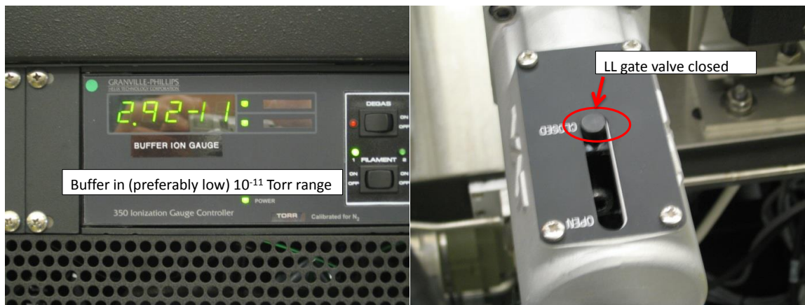
Figure B.12. The buffer chamber pressure must be sufficiently low, and the LL gate valve must be shut before the gate valve to the growth chamber can be opened.
