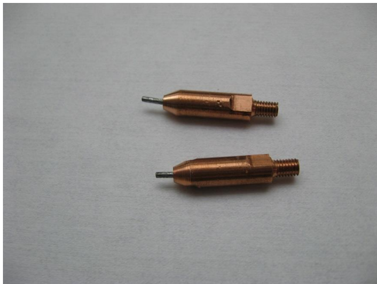
Figure 2.15. Homemade molybdenum tips for spot-welding MBE components.
