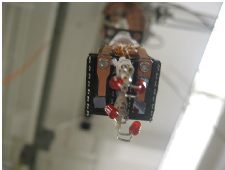
Figure H.3. Copper headers mounted on the tail. Care should be taken when removing the radiation shield to not bump the LEDs with the shield.
