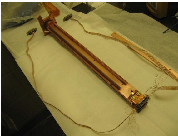
Figure 3.11. Tail after cleaning with Brasso metal polish, toluene, acetone, and methanol.
