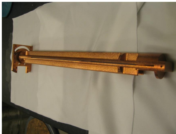
Figure 3.10. Tail after etching in 1:1 water:nitric acid.
