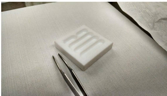
Figure G.5. Homemade teflon inserts used to sonicate multiple samples in parallel.
