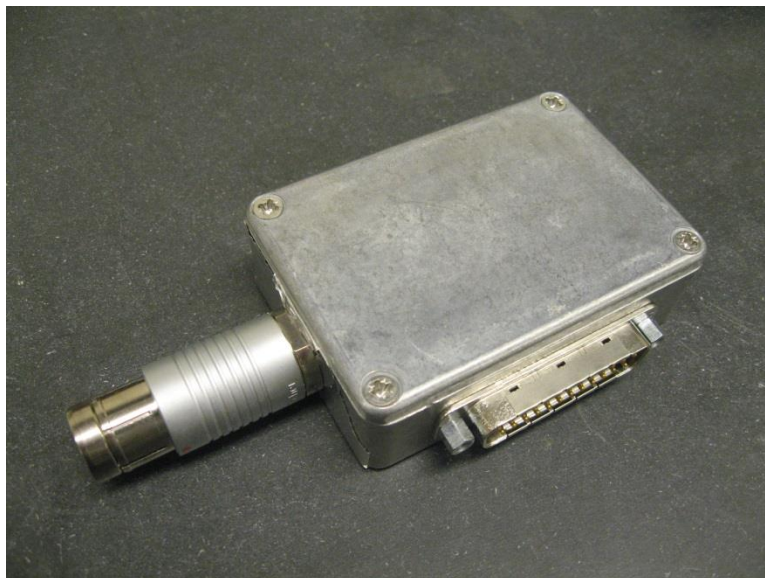
Figure 3.8. Homemade filter box that couples a D-SUB 25 cable to the Fischer connector on top of the fridge.
