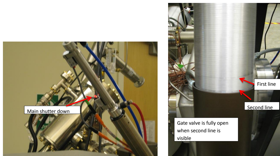
Figure B.13. The main shutter should also be down before the gate valve is opened (left). The gate valve is fully open when the second line on the arm is visible (right).
