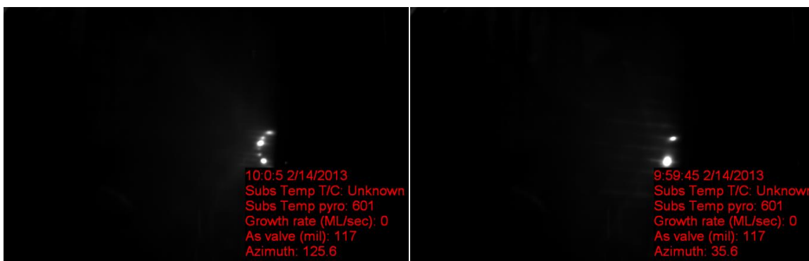
Figure B.8. Comparison of the 2\times reconstruction (left) and 4\times reconstruction (right) as seen on the RHEED screen.
