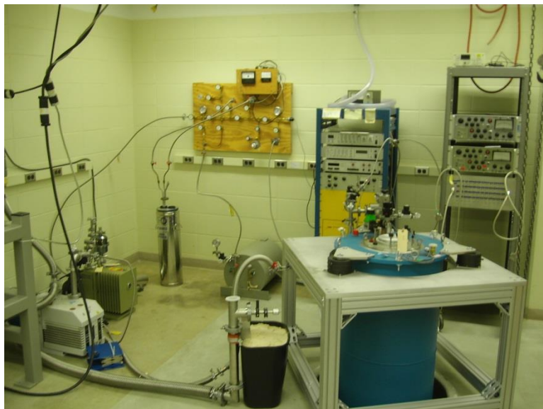
Figure 3.4. Dewar, magnet, and stand in place at end of the initial construction phase.
