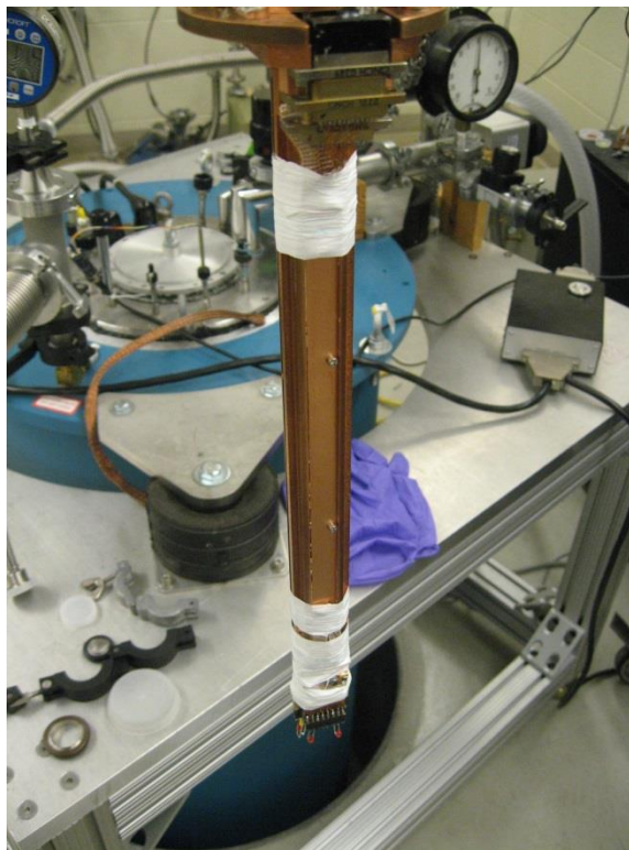
Figure 3.13. Finished tail mounted on the mixing chamber.
