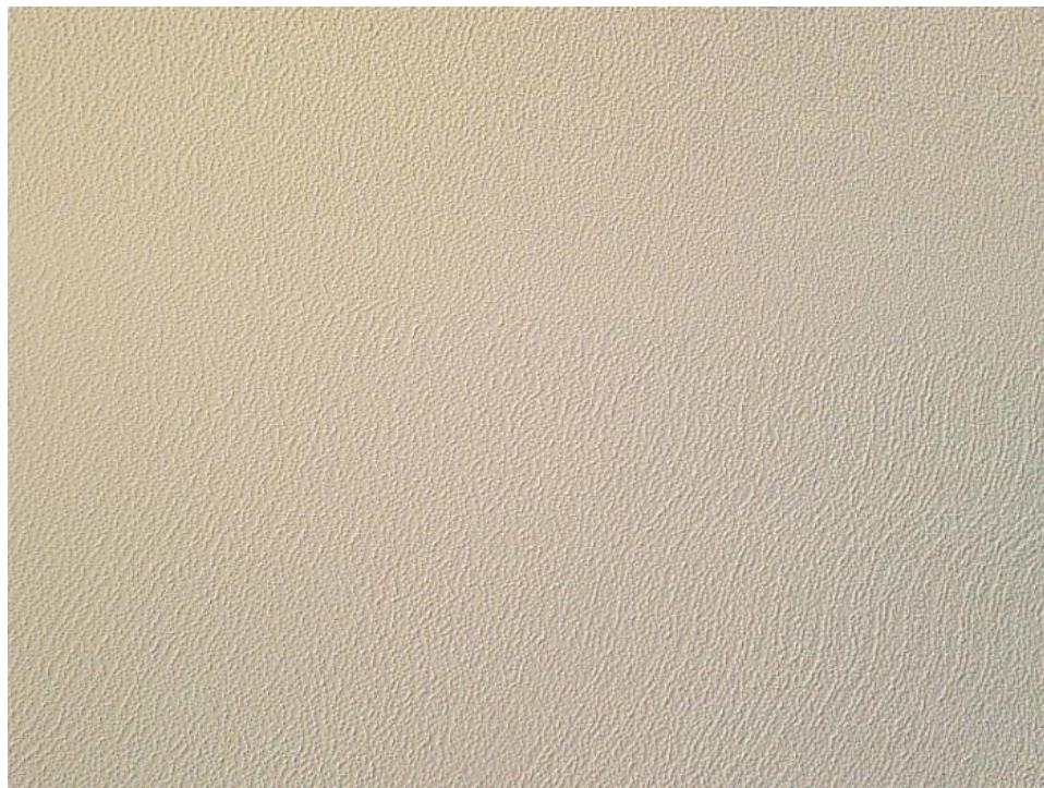
Figure B.27. Nomarski phase contrast micrograph of a hazy wafer. The field of view is \sim 2.5 mm wide.
