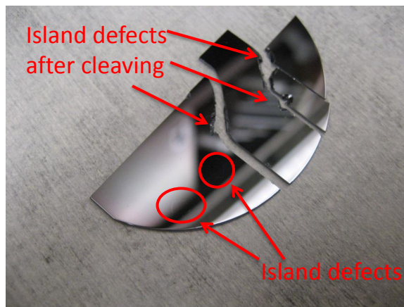
Figure 2.18. Wafer with so-called “island defects” after cleaving. Two defects (circled) away from the cleave lines as well as a few defects along cleave lines are called out in the figure.
