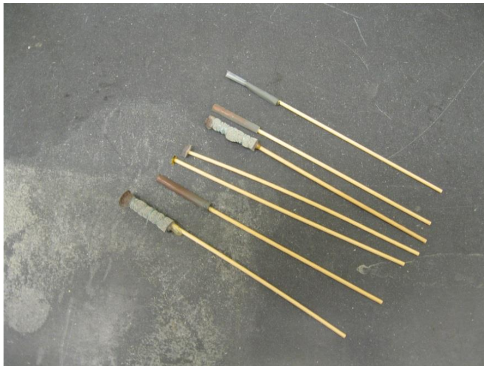
Figure H.4. Homemade sandpaper tools for cleaning copper oxide off of small pieces. 2000 and 3000 grit sandpaper is glued to wooden sticks with quick set epoxy to aid in cleaning small copper pieces such as the headers.
