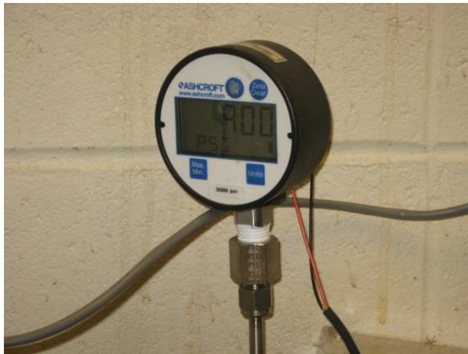
Figure E.2. Pressure gauge behind the computer showing the “P impure” reading.
