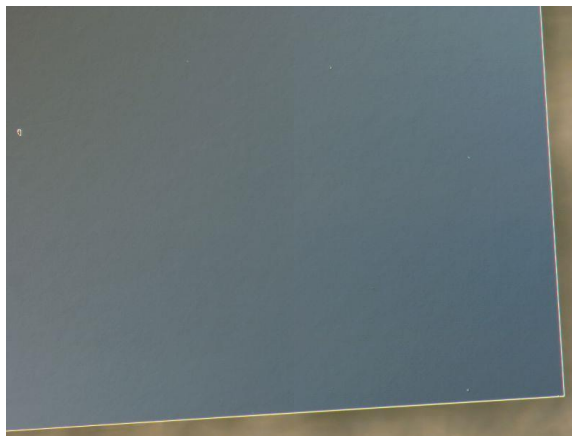
Figure G.6. Surface of wafer after gallium removal and sonicated cleaning. Field of view is \sim 2.5 mm wide.
