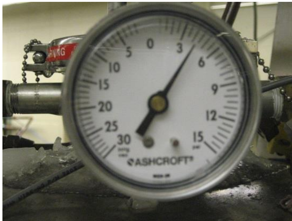
Figure E.4. Liquefier dewar pressure. Do not let this pressure exceed 6 psi if the liquefier is running.
