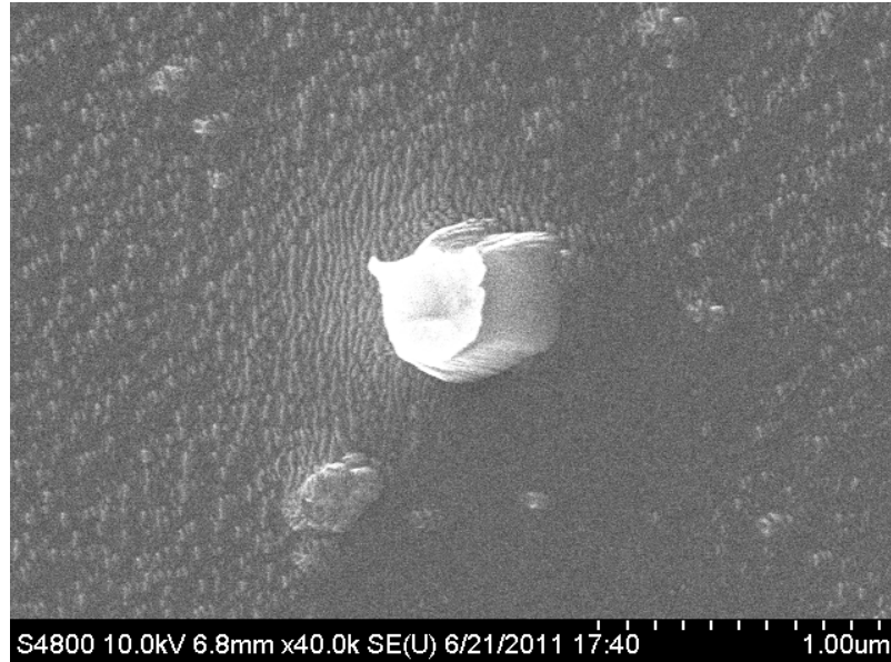
Figure 3.3 : Silicon surface after irradiation with 200 eV Ar + ions at 10° to a fluence of 6E17 cm -2
