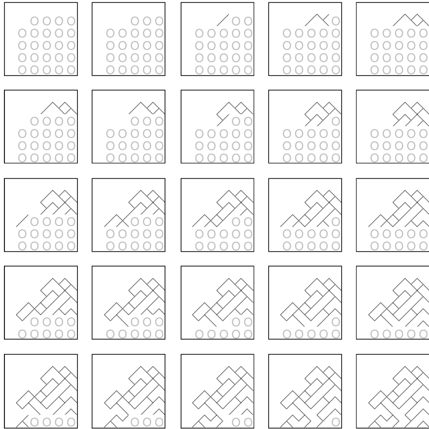
Figure 4.1. Snapshot of the example tiled image after each tiling iteration. The 'O' symbols, which are the nonterminal open symbols, and the border are shown for illustration purposes only.
