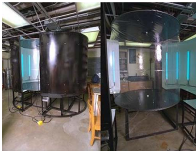
Figure 2.2. The Shepson group all-Teflon photochemical reaction chamber at Purdue University.
