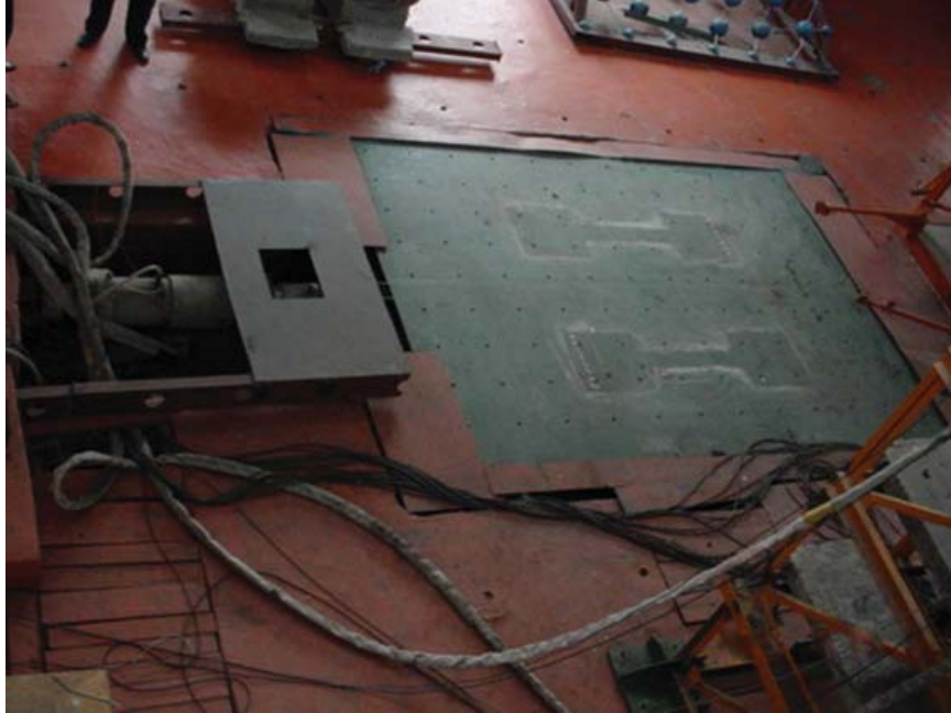
Figure 2.8: Shake table located at HIT
