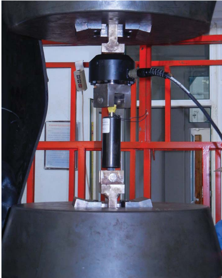
Figure 2.24: MTS loading frame with MR damper and load cell attached at HIT
