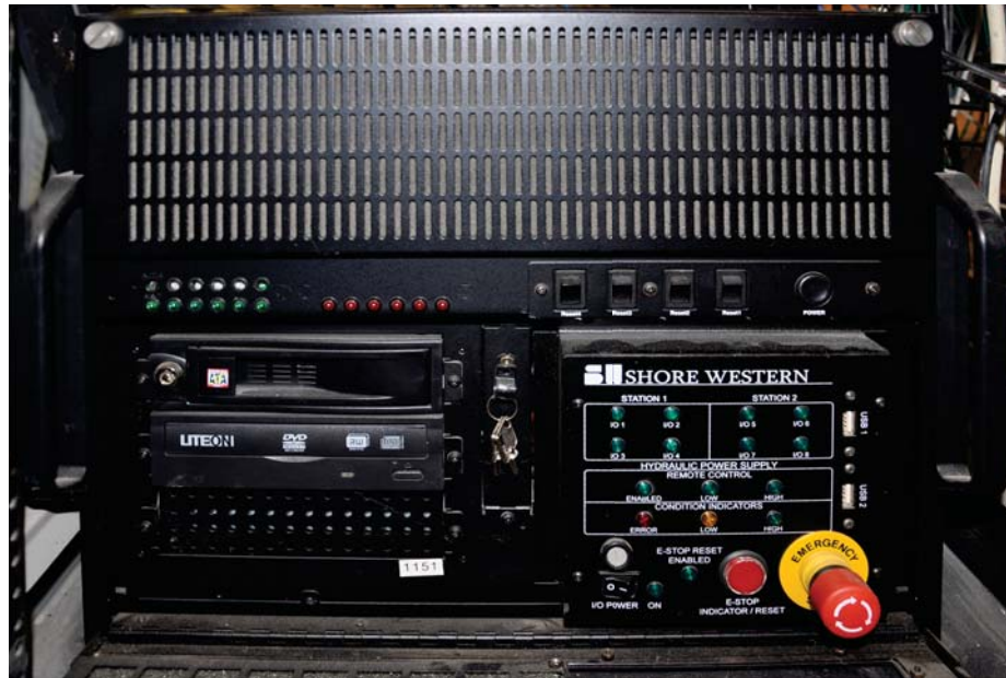
Figure 2.26: Shore Western SC6000 controller
