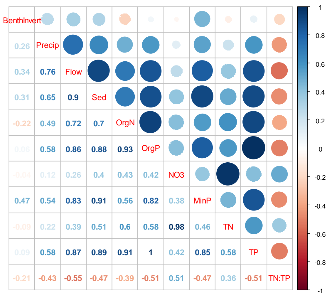
Figure 3.13 Correlation matrix for the annual loads regression model. The larger the circle the greater the correlation. Blue colors indicate positive correlation and red colors indicate negative correlation.
