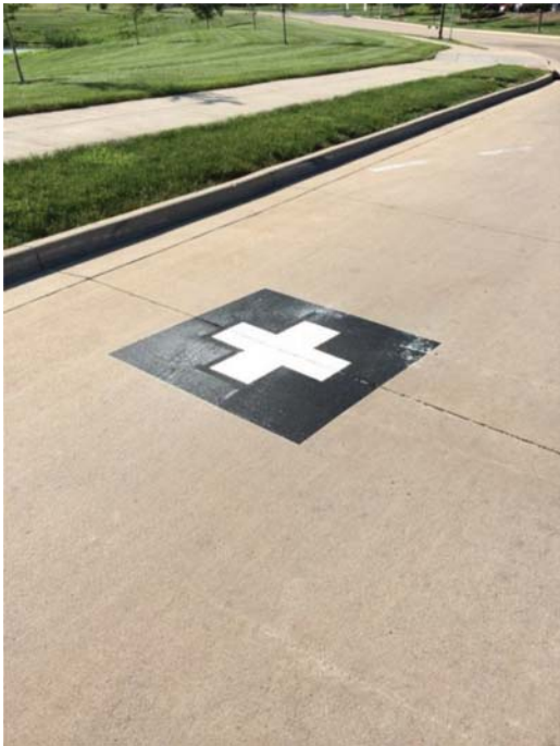
Figure 3.4 Painted target with cross pattern.
