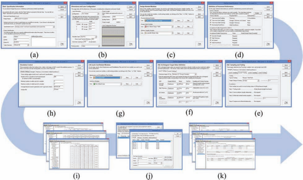
Figure 3.1 PavSpec workflow: (a) basic specification information; (b) dimensions and lane configuration; (c) design-related modules; (d) definition of pavement performance; (e) AQC sampling and testing; (f) AQC as-designed target value definition; (g) life-cycle cost-related modules; (h) simulation control; (i) results—pay factor matrices and LCCs (as-designed); (j) as-constructed AQCs; (k) overall pay factor and LCC (as-constructed).
