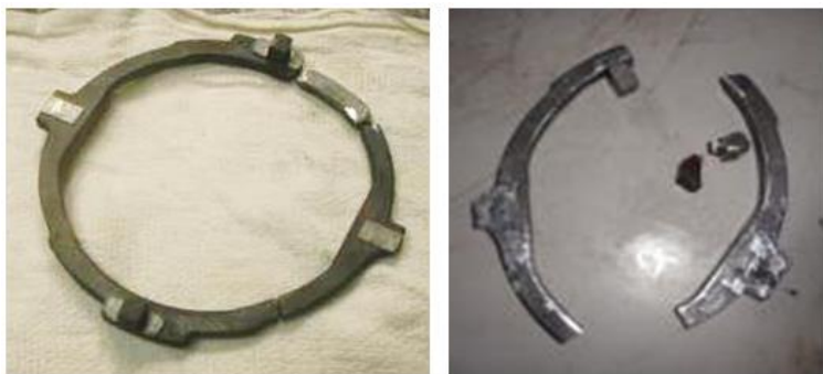
Figure 2: Two broken OC
