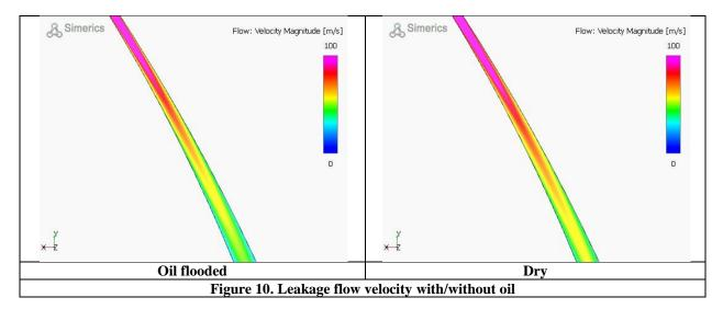
Table 2 shows the major performance difference when compressor run dry or with oil flooded. The results show a gradual increase in refrigerant mass flow rate, a gradual decrease in power consumption, and a significant temperature reduction when the oil contents in compressor increases. Those trends match the expected oil cooling and sealing effects.
