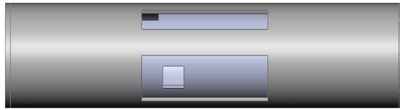
(a) Intake port (smaller port) of the left chamber is open, the piston moves from left to right. Expanded working fluid in the right chamber is discharged to the condenser (wider port).
