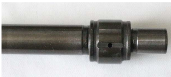
Figure 10: Wear of the crankshaft of the normal
