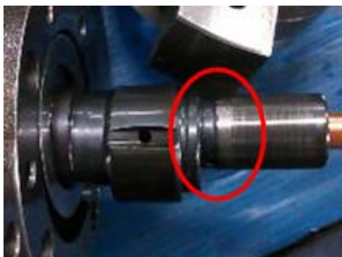
Figure 2: Photo of the wear of the crankshaft
