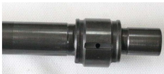
Figure 11: Wear of the crankshaft with short main bearing
