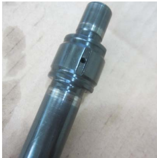
Figure 13: Wear of the crankshaft with small clearance bearing
