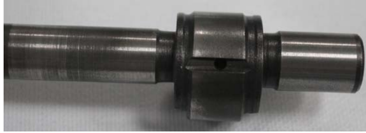
Figure 12: Wear of the crankshaft with small diameter of crankshaft
