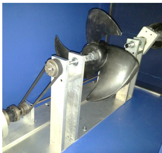
Figure 2: Laboratory facility for measuring air side heat transfer coefficients of a rotating fan blade
