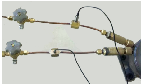
Figure 2: Compressor pressure pulsation test bench
