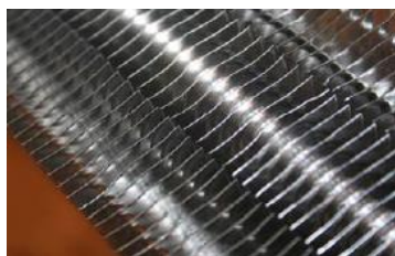
Figure 8: Cut fins to reduce heat conduction from warm to cold tube rows
