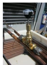
Figure 9: Needle valve to speed up optimization of capillary tube and charge
