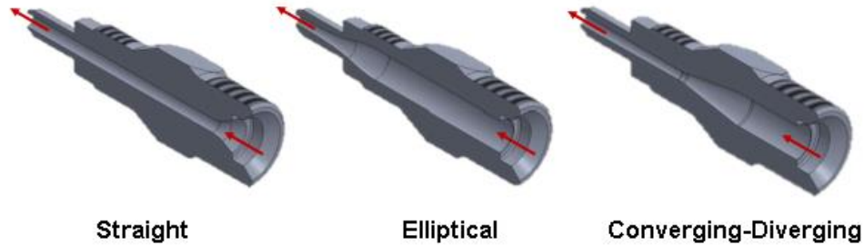
Figure 4: Nozzle types used with the Viper Expander.
