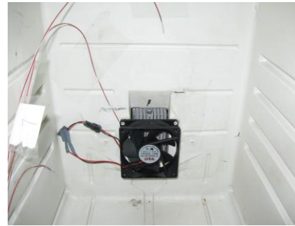
FIG 1. The system assembly of a thermoelectric cooler FIG.2 The arrangement of 3 testing points for dynamic temperature monitoring
