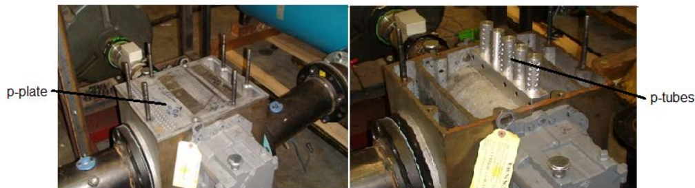
Figure 9: Comparison of prototype setup of perforated tubes (p-tubes) with a perforated plate (p-plate)
