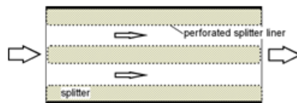
Figure 2b: Principle of an absorptive silencer
