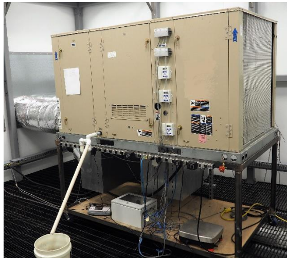
Figure 3. 5-ton RTU used to test automated fault detection and diagnostics system installed in psychrometric chambers.
