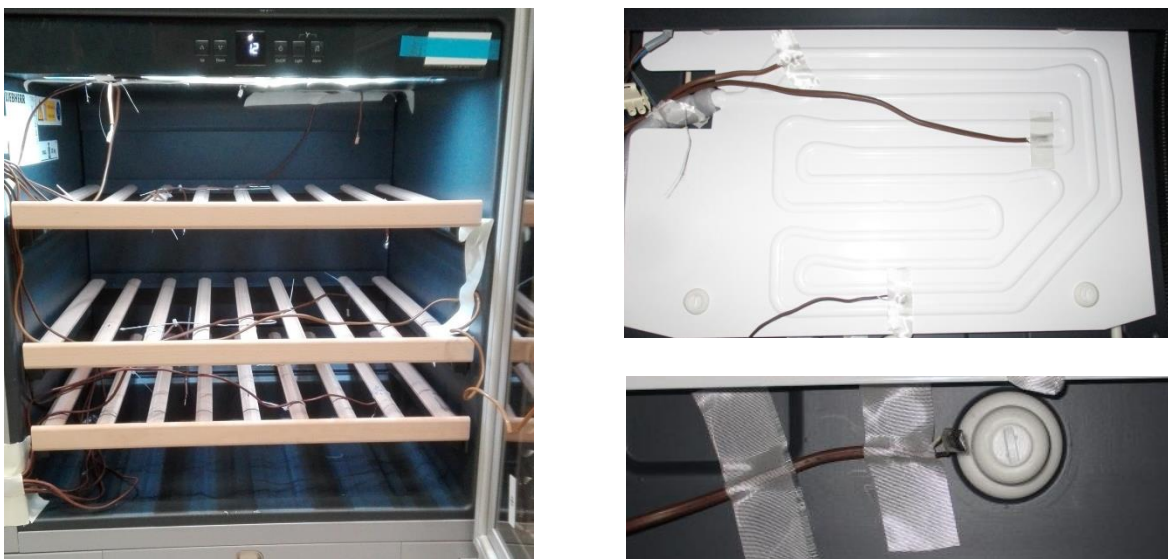
Figure 2: Experimental setup – compartment, evaporator and close-up view of a measurement point
