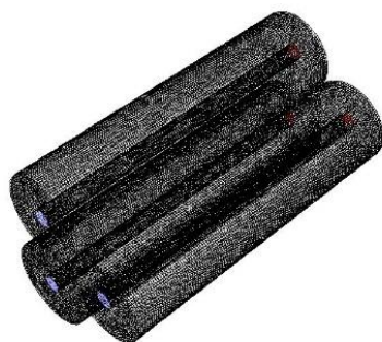
Figure 3: The pipe arrangement method
