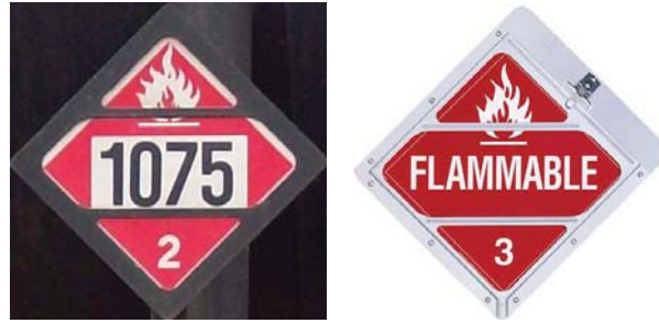
(a) An example of a hazmat sign used for a train tank car. (b) An Example of a hazmat sign used for a truck trailer.
