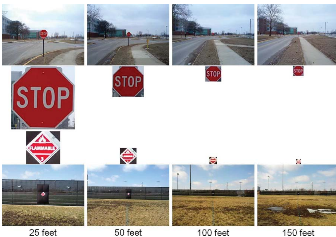
Fig. 3.21. Examples of bounding box images for a typical STOP sign and a hazmat sign at the same distance 25, 50, 100, and 150 feet.
