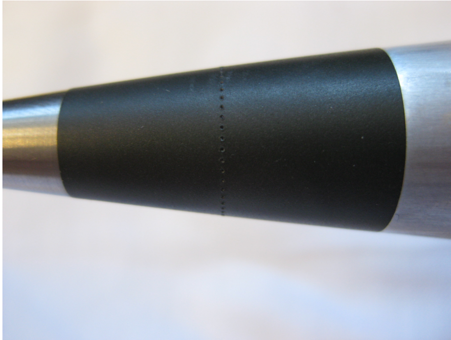
Figure 3.10.: Torlon section and 50-dimple case.
