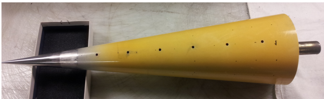
Figure 3.12.: 7^\circ half-angle Heat Transfer Cone with temperature-sensitive paint applied to the frustum. The sensor ports are visible as the larger black dots along a single ray. The smaller black dots were used as reference points.
