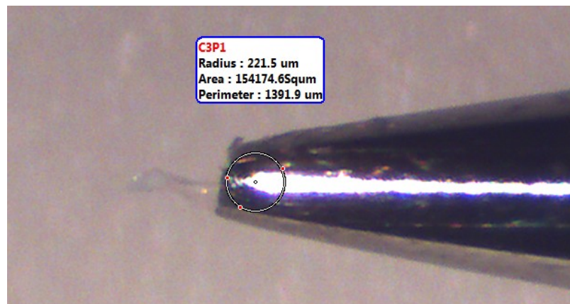
Figure 3.9.: Nosetip of 7° half-angle Crossflow magnified 20 times.
