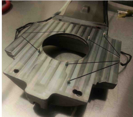
Figure 4.5. Sensors installed on the bottom half of the swashplate (top swashplate not shown).
