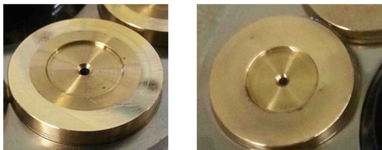
Figure 4.16. Photograph of a slipper following run-in (left) and following full testing at six operating conditions (right).
